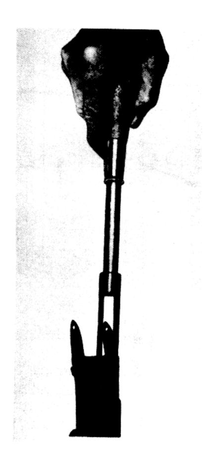
Removing flexible plunger head assembly
